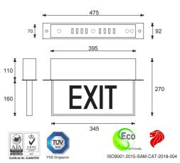
... is designed to be slim and lightweight, low EMI and specially equipped with a customised proprietary Hybrid IC and a very high efficiency current feed push-pull sine wave inverter, to fully utilise the battery power and to prevent the frequent blackening of the tube.
