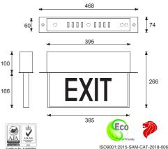
... is designed and specially equipped with a customised proprietary Hybrid IC and a very high efficiency current feed push-pull sine wave inverter, to fully utilise the battery power and to prevent the frequent blackening of the tube. Compact and lightweight. Easy and fast installation with the thumb-press quick lock fastening system cuts down installation/maintenance time drastically.
